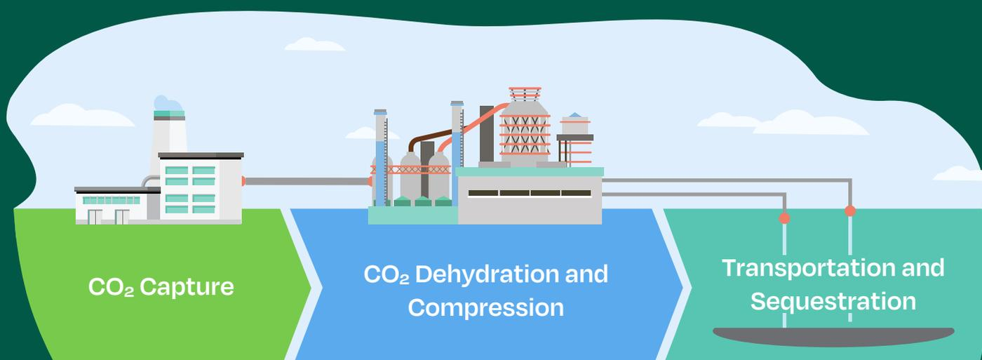
Carbon capture and sequestration, or CCS, is the process of capturing carbon dioxide (CO<sub>2</sub>) before it is emitted to safely and permanently sequester it in proven and secure storage areas deep underground.
