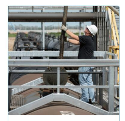
The nimbleness of our logistics and distribution facilities is enabled by well-positioned facilities and a fleet of transportation assets. Here, a shipping technician loads UAN into a railcar at the Port Neal Nitrogen Complex.
